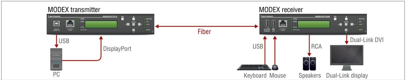
Any transmitter can be connected to any receiver: the DisplayPort input is converted to Dual-Link output automatically by MODEX transmitting the USB KVM devices signal as well.
