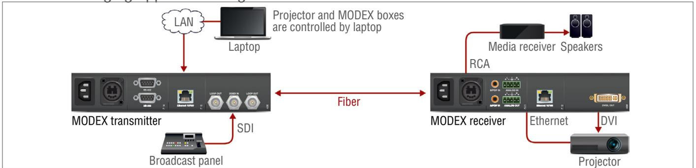
SDI transmitter connects directly to the DVI receiver. The transmission is format free; MODEX sends the video pixels regardless of the video format.
