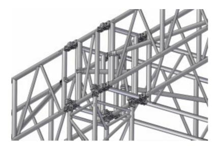
The procedure follows closely the three ways corner with vertical forks solution, but before closing by nuts or bolts all the vertex', fix QL52 truss fixed to the quadrilater base using three forks (two males and one female or two female and one male in order to connections previously realized). This system's purpose is locating the forks to lodge the tower.
