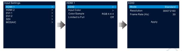
Step 8 Rotate the knob to select Apply and press the knob to complete the standard resolution settings.
