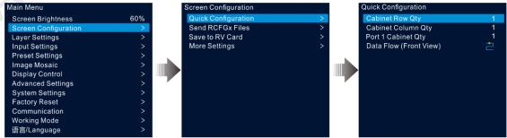
Step 3 Rotate the knob to select Port 1 Cabinet Qty to set the quantity of the cabinets loaded by Ethernet port 1.
