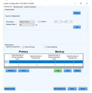
Step 8 Repeat Step 6 and Step 7 to complete the backup settings for other Ethernet ports.
