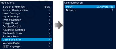
Step 2 Rotate the knob to select **Mode** and press the knob to confirm. Rotate the knob again to select the desired mode and press it to confirm.
