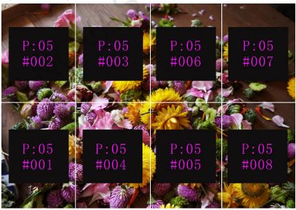
P:05 indicates the Ethernet port number of the sending device. #001 shows the number of the cabinet loaded by the Ethernet port.
