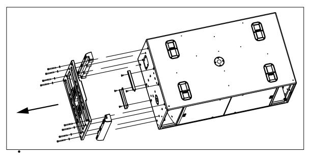
• Remove the four screws on each side of RS18.
