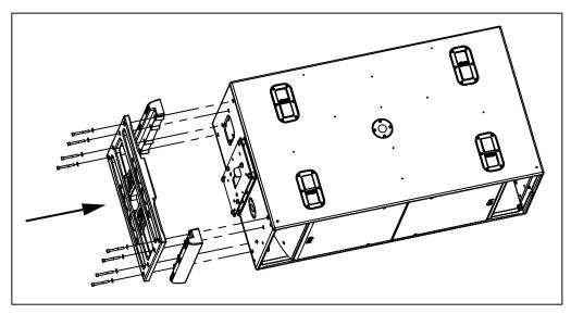
INSTALLING CARPETED RS18 RIGGING PLATES
