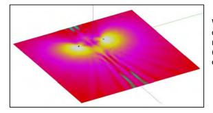
When using few cabinets, minimizing overlap can only be achieved with directional devices by rotating the subwoofers 30° to 45° outwards (rotating an omnidirectional subwoofer makes no difference in the coverage pattern).
