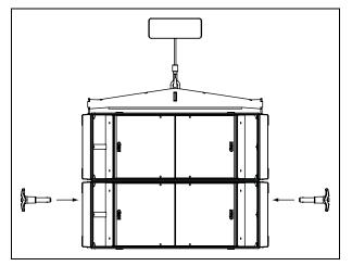
• On both sides, push the top RS18 sliding connecting plate all the way downwards into the second RS18 rigging system
