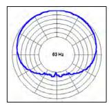
Gradient subwoofers can provide up to 15 dB front to rear average attenuation (Please refer to Ray Sub technical note for in-detail explanation on gradient subwoofers).
