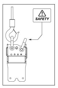
• Secure bumper with secondary safety steel.
