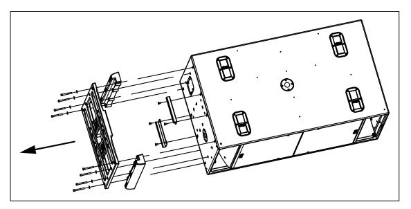
• Remove the four screws on each side of RS18.
